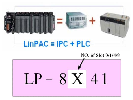
The LinPAC-8x41 model type is ruled as LP-8x41, as shown in the above figure. The Second number shows the slot numbers coming with the main controller unit. Currently, we provide three types of  $0 \cdot 1 \cdot 4$  and 8 slots. The last number demonstrates the application platform. 1 stands as the Master controller and it means that the user needs to design the application program by themselves.
